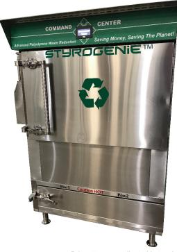
Briquettes are collected in two bottom trays. Between 1400 and 1800 soiled trays are easily loaded and processed daily. Briquette below contains over 600 densified polystyrene trays.
