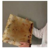
Briquettes measure approximately 16" X 20" and are between 2"-4" thick, weighing 12-15lbs on average.
